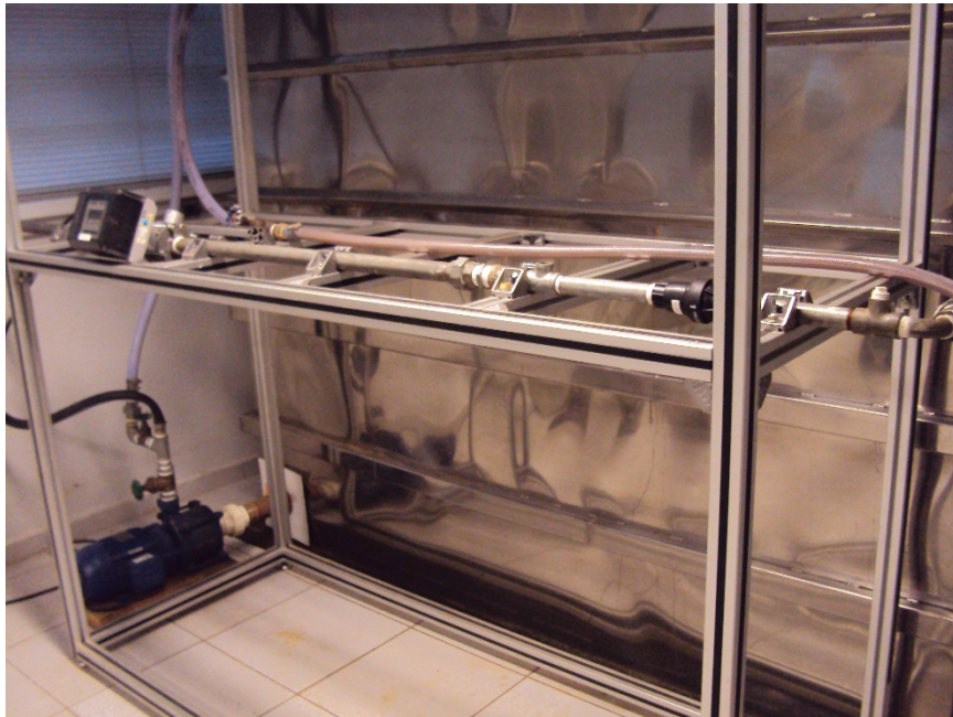
Testing bench for pressure-regulating valves and Venturi injectors
