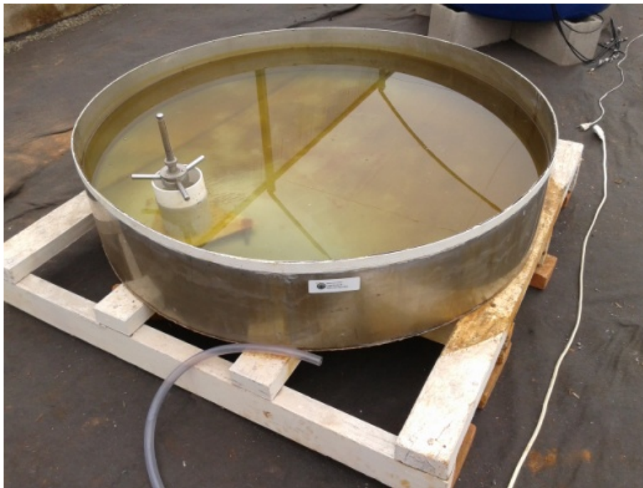
Figure 1. Experimental setup to measure surface (0.05 m) dielectric permittivity ( K_a ) using TDR, lysimeter and auxiliary column used to monitor the water level inside the lysimeters (A); Class A pan used to measure atmospheric demand (B)
