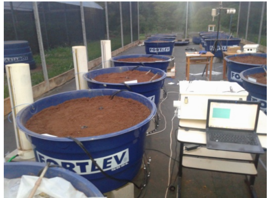
Figure 1. Experimental setup to measure surface (0.05 m) dielectric permittivity ( K_a ) using TDR, lysimeter and auxiliary column used to monitor the water level inside the lysimeters (A); Class A pan used to measure atmospheric demand (B)
