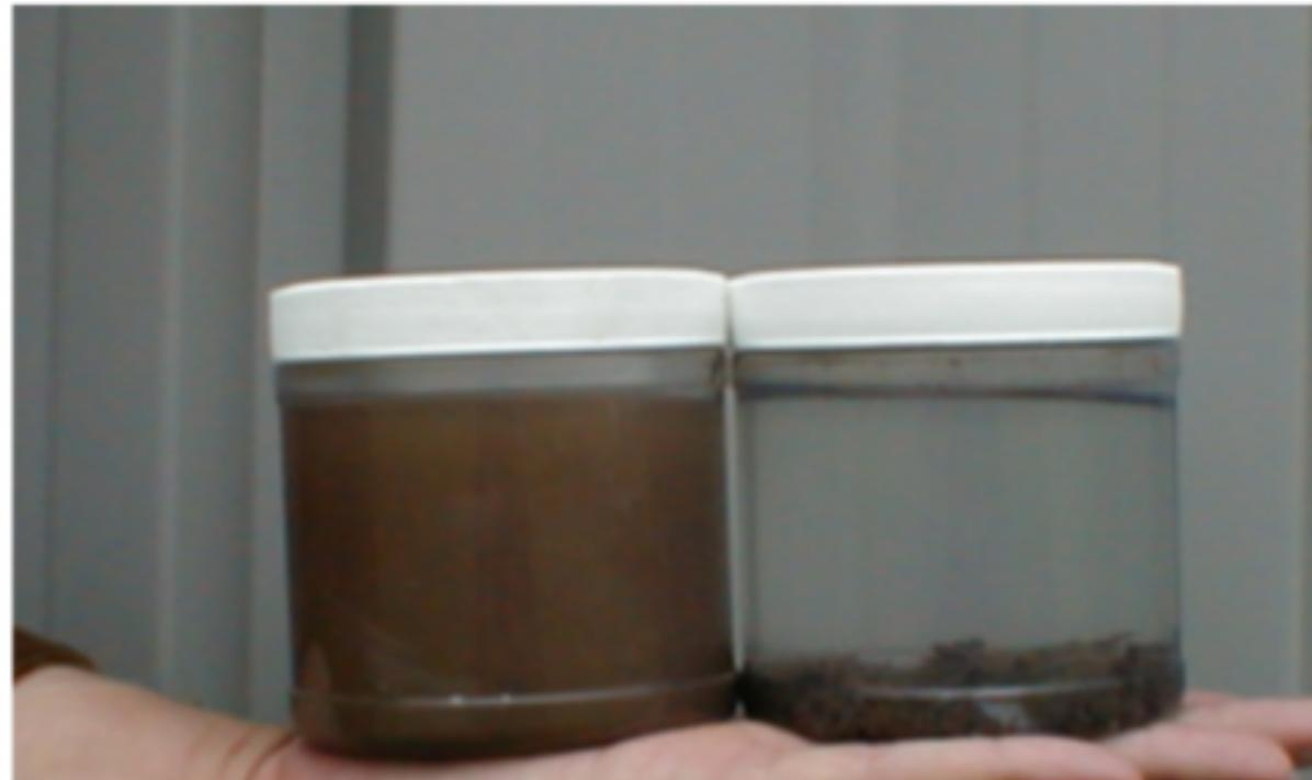
TSS before and after the use of a clarification polymer for flocculation (source: cfmwi, 2013)
