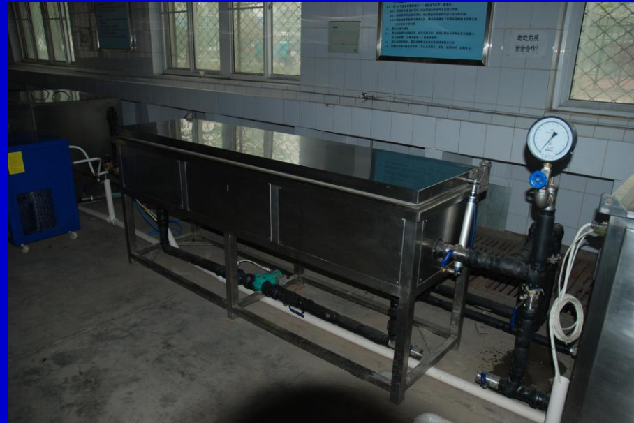
Resistance to hydraulic pressure at elevated temperature (60°C) for Emitters
