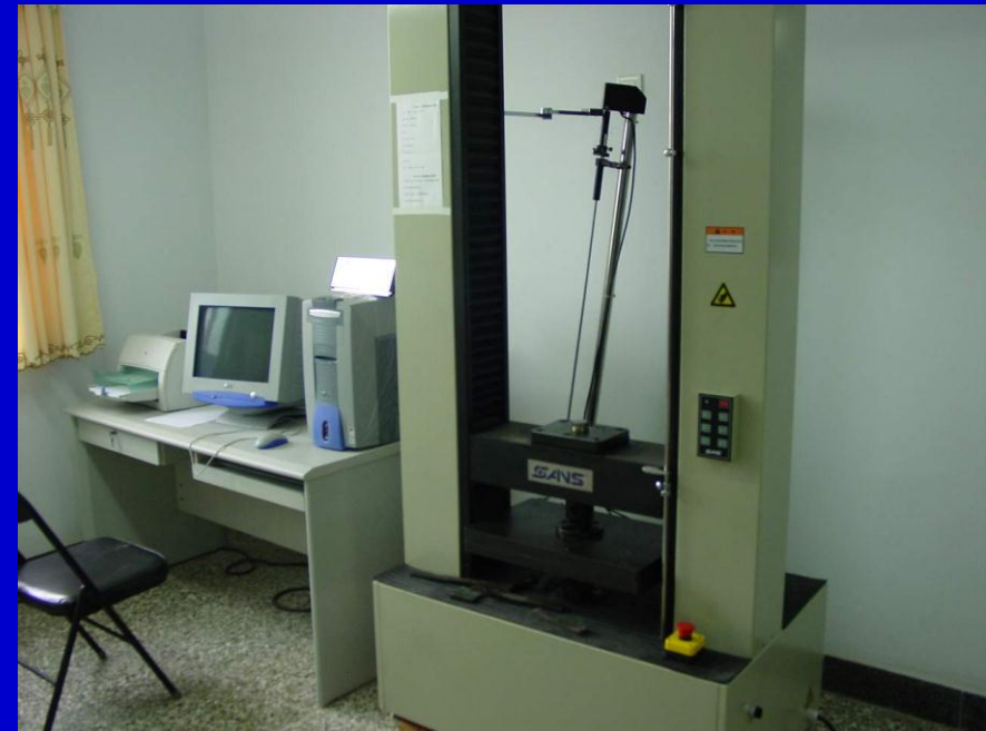
Universal computer-controlled electronic tester
