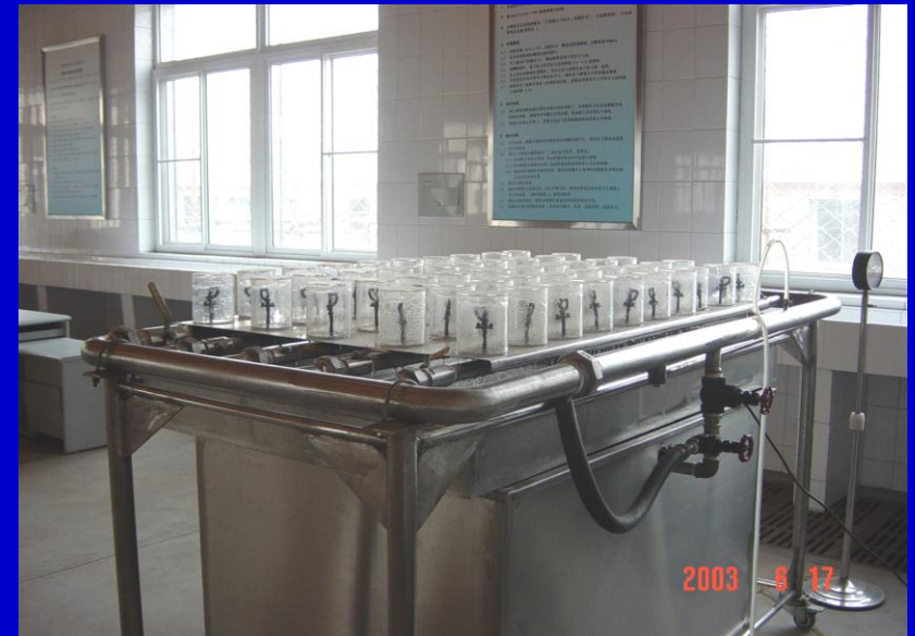
Test equipment for micro-sprayer durability
