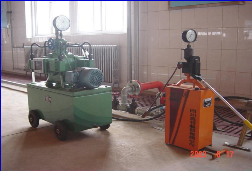
Test equipment for hydraulic performances of metal pipe
