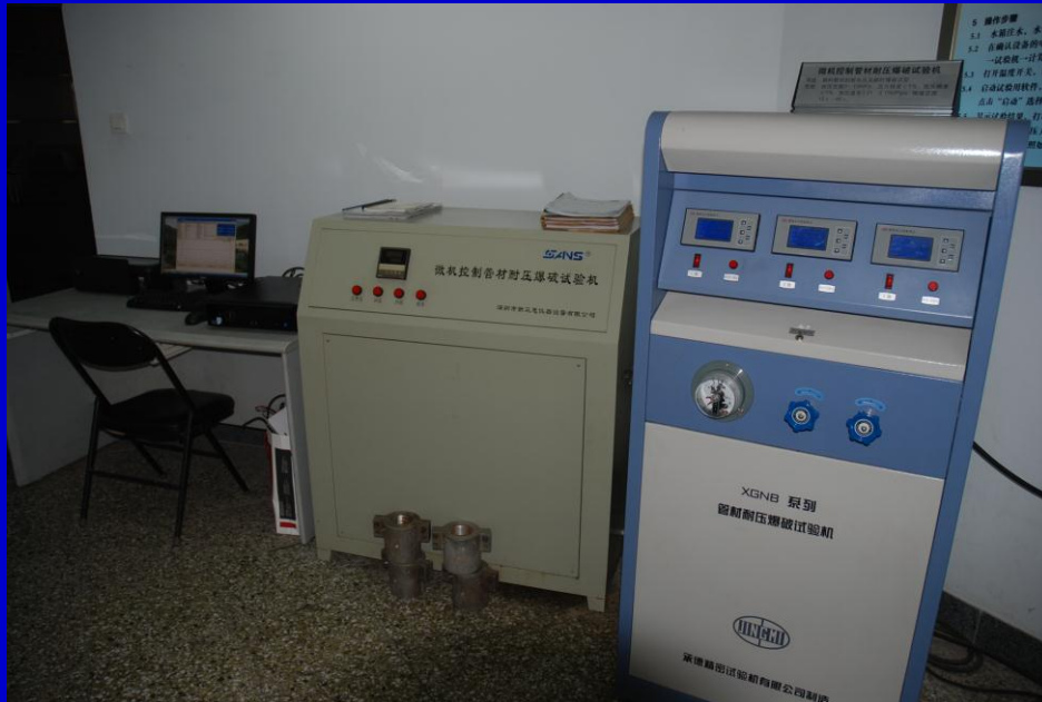
Tester for durability and blasting of pipes
