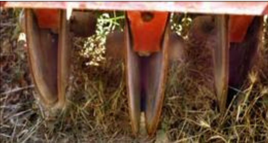
Double disc seeder opener
